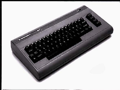
■ The C64 CPU and keyboard unit in its original form, owing something to those P500 days.
